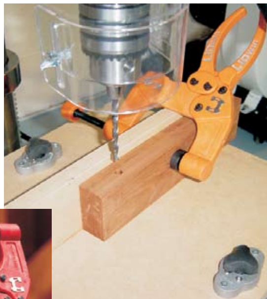
Photo.3: This setup uses two MagJigs (centre left and bottom right) to secure the jig on a drill press table and an X4 to lock the workpiece in position
