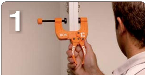
**Step 1:** Now that we have established that the clamping width is 32mm, hold the clamp between the cupboards with a width of 33mm or more.
