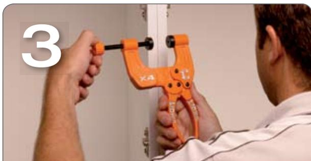
**Step 3:** Open handles to remove clamp from cupboards. Slowly wind the adjustment knob 360 degrees clockwise 1 – 2 times. (The amount of times you need to turn the adjustment knob depends on the rigidity and clamping strength required).
