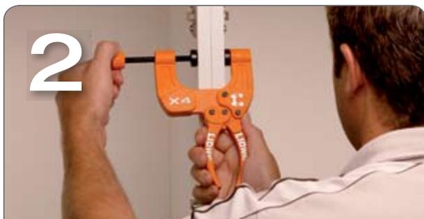
**Step 2:** Slowly wind the adjustment knob towards the two cupboards. (The clamp width should be 32mm touching either side of the carcass).
