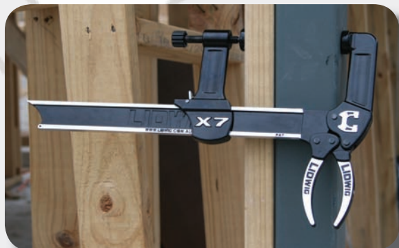
Photo. 2 The Lidwig X7 clamp with up to 310mm capacity
